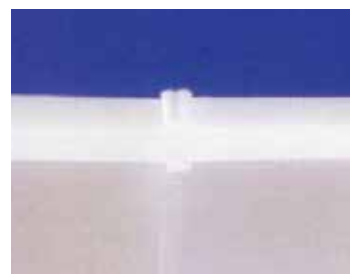
溶着接合部 Photograph of butt Fusion joint
