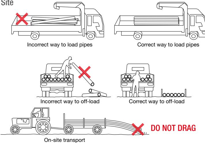
**NOTE:** The impact resistance and flexibility of PVC and especially CPVC pipe are reduced by lower temperature conditions. The impact strength for both types of piping materials will decrease as temperatures approach 32°F (0°C) and below. Extreme care should be taken when unloading and handling pipe in cold weather. Dropping pipe from a truck or forklift can cause damage. Methods and techniques normally used in warm weather may not be acceptable at the lower temperature range.
