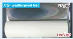
Weatherproof test (Impact strength) 400 350 Crack height(cm) UVS-VP PVC Pipe(VP) 300 250 - Strengthned PVC Pipe(HI) -200 100 20% 10 Equivalent years of outdoor exposure (years)
